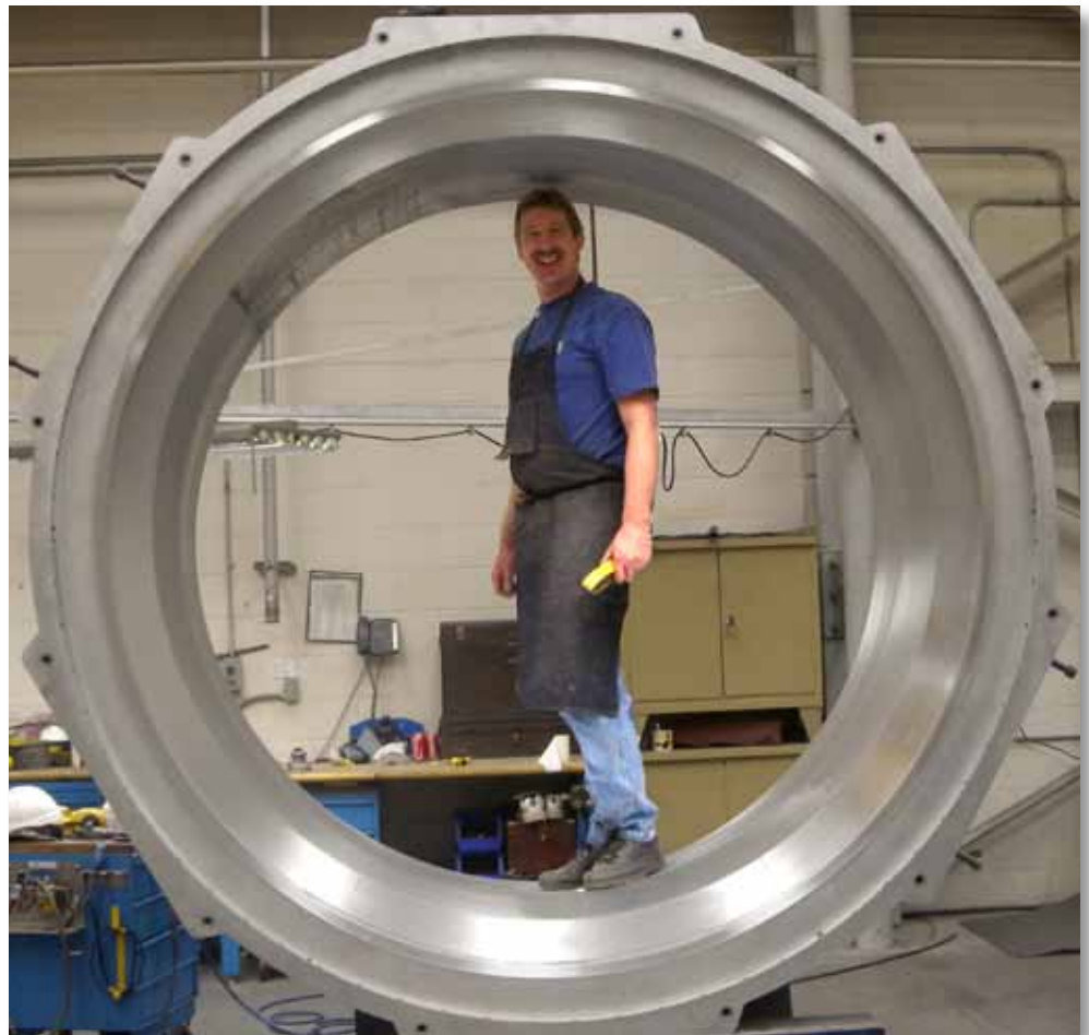
Bill Smits, a bench hand at Paragon D&E, sands a mammoth aluminum mold part. Smits spent about 200 hours sanding down rough edges on the part, which will eventually be used to create a carbon fiber airplane engine shroud.
