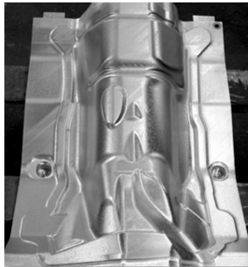
This is the mold part that Seaway Pattern produces for the transmission tunnel, which is responsible for the hump in the middle of the floorboard of many cars.
