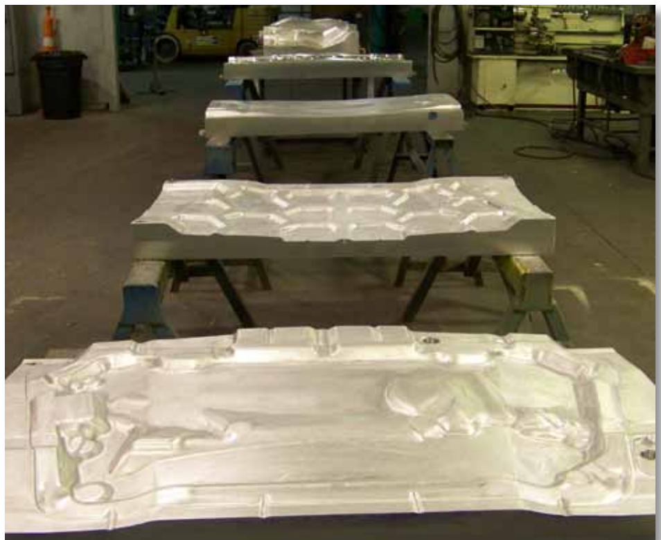
Molds that are destined to make the insulation batting found under the hood of a car are lined up on horses at Seaway.
