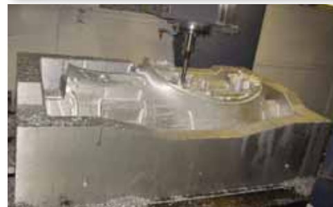
Above: Clinton's Duramold 2000 stock is a key part of this prototype instrument panel mold. Below: One-half of a fuel tank production mold.
