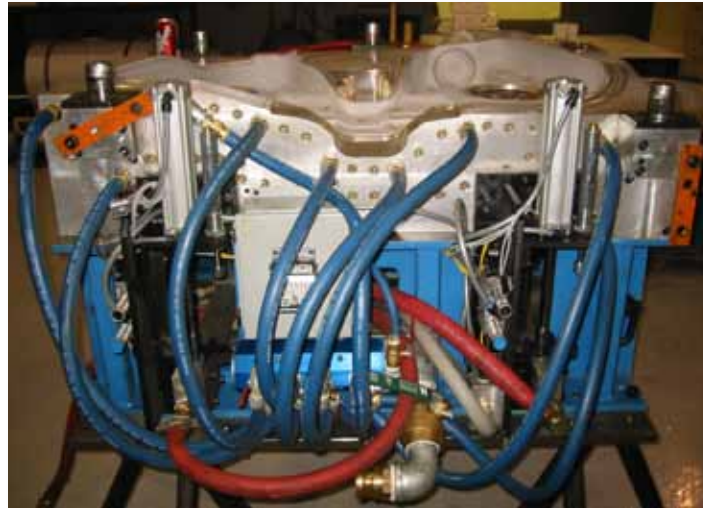
Above: Clinton's Duramold 2000 stock is a key part of this prototype instrument panel mold. Below: One-half of a fuel tank production mold.
