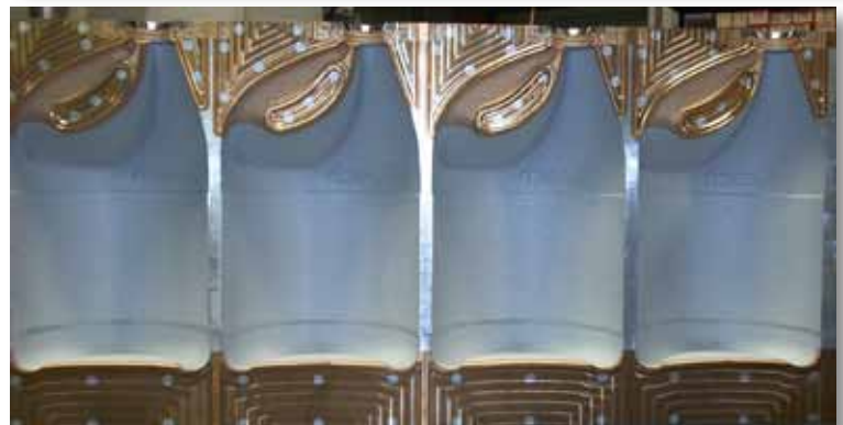
Monroe Mold turns Clinton Aluminum material into bottle-making molds for the personal-care and medical industries, among others.
