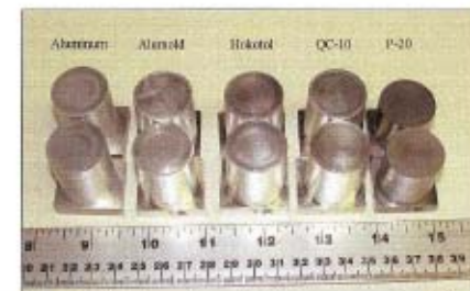
Figure 9. Image of the five alloy sets. This image was taken after the completion of the cyclic compression tests.
