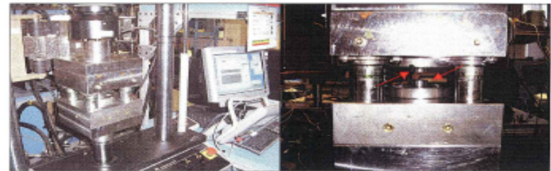
Figure 8. Compression frame and test jig fixture employed in the test of the five alloys. The arrows highlight the location of the test specimens.
