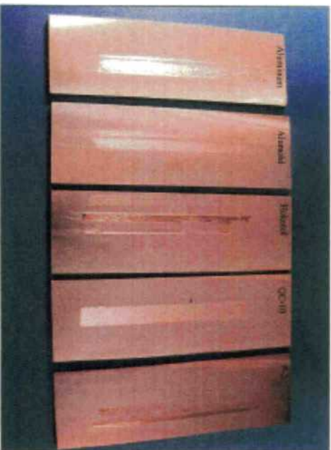
Figure 2. Image of the five platens after the linear abrasion test.
